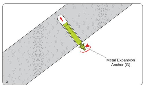
Insert the metal expansion anchors (G) and hammer them into the drilled holes. Make sure to leave a portion of the anchors outside of the concrete. Then, take off the washers and the nuts on the anchors by using a socket wrench.
