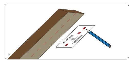
Using wall marking template (B), mark on the center of the stud the locations of where you want to mount the ceiling adapter.
