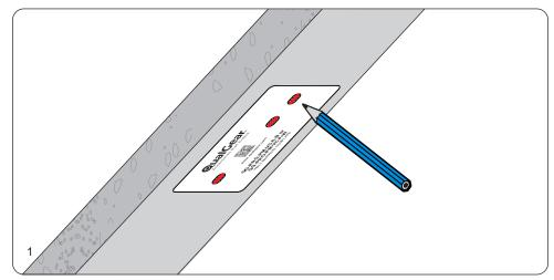
Using wall marking template (B), mark on the concrete the locations of where you want to mount the ceiling adapter.
