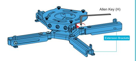
Depending on your projector, adjust the extension brackets on the projector mount (A) accordingly by using Allen Key (H).
