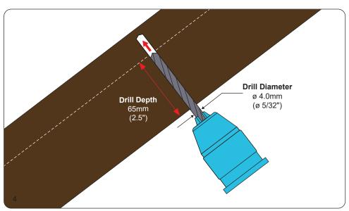
Using a power drill and a 5/32" wood drill bit, drill holes of 5/32" (4mm) diameter, and 2.5" (65mm) depth at the marked locations.
