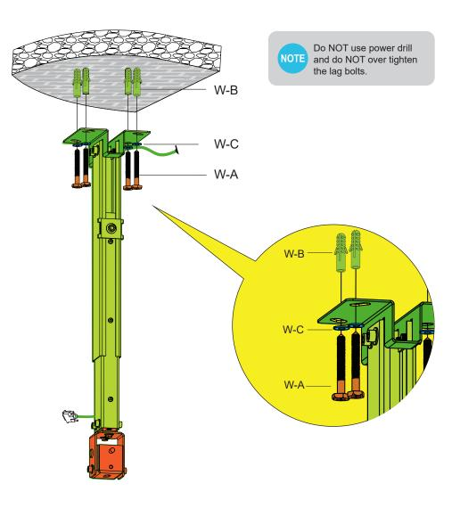
Place concrete anchors (W-B) in each hole. Tap each anchor flush with the ceiling surface using a hammer. Mount the ceiling plate and tighten with the lag bolts (W-A) and washers (W-C) using a socket wrench.
