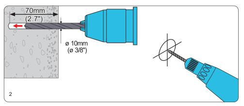
Using a power drill and a 3/8" masonry drill bit, drill mounting holes of 3/8" (10 mm) diameter and 2.7" (70 mm) depth at the marked locations in the previous step.
