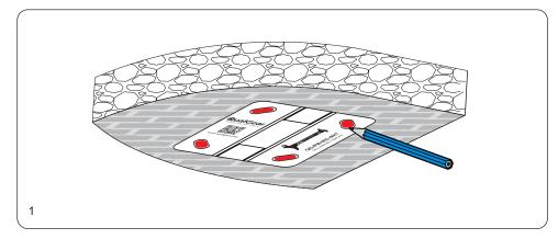
Hold the marking template provided against the ceiling where you want to install the projector, mark four holes for drilling.
