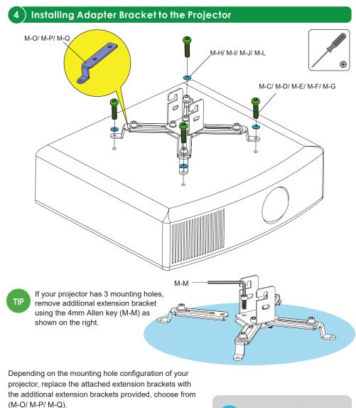
Then, place the projector bracket as close to the center of gravity of the projector as possible, align the holes of the extension brackets over the mounting holes of the projector. Select the appropriate screws (M-C/ M-D/ M-E/ M-F/M-G) and washers (M-H/M-I/M-J/M-L) according to the mounting holes of your projector, and tighten the screws using a screwdriver.
