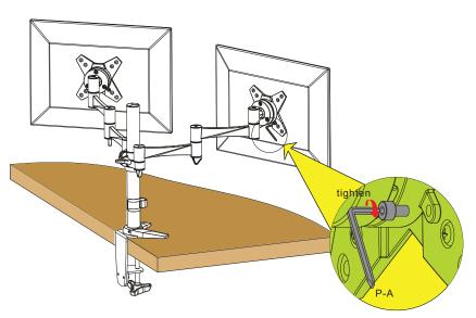
Attach the VESA plate to the mount with the retained screws from Step #2 (see page 3) and tighten them using a 3mm Allen Key (P-A).
