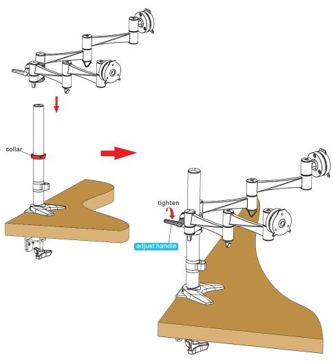
Insert the articulated arm assembly into the pole until it touches the collar. Then tighten the adjust handle.
