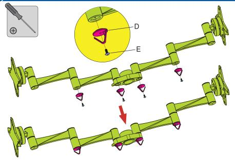
Install cable clips with the provided screws using a Philips screwdriver.
