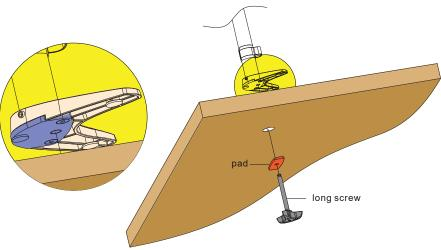
Insert the long screw into the base plate through the hole and pad (P-D) as shown above. Then tighten the long screw to hold the mount securely.
