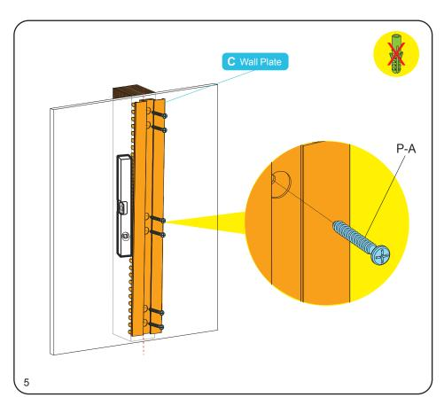
Mount the wall plate (C) and tighten it with the provided lag bolts (P-A) using a proper Phillips screwdriver.
