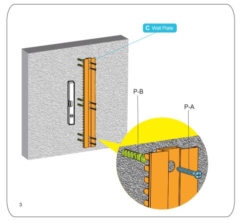
Place concrete anchors (P-B) in each hole. Tap each anchor flush with the wall using a hammer. Using a proper Phillips screwdriver, mount the wall plate (C) and fasten them with the provided lag bolts (P-A).
