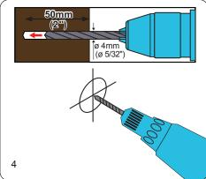
Using a power drill and 5/32" drill bit, drill pilot holes of 5/32" (4mm) diameter and at least 2" (50mm) depth.
