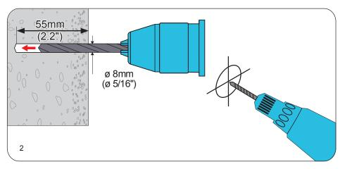
Using a power drill and a 5/16" masonry drill bit, drill mounting holes of 5/16" (8 mm) diameter and 2.2" (55 mm) depth at the marked locations in the previous step.
