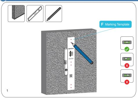
Hold the marking template (F) provided against the wall where you want to install your AV equipment, mark six holes for drilling.
