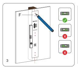
Using the marking template (F) provided, mark six holes for drilling on the centerline of the stud.
