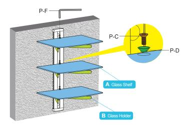
Attach the glass shelves to the glass holder using the plastic bushes (P-D), screws (P-C) and Allen Key (P-F)."
