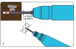
Using a power drill and 5/64" drill bit, drill pilot holes of 5/64" (2mm) diameter and at least 1" (25 mm) depth.
