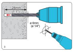
Using a power drill and 1/4" drill bit, drill pilot holes of 1/4" (6mm) diameter and at least 1.1" (28 mm) depth.
