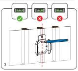
Using the wall mount as a template, mark two holes for drilling on the centerline of the stud.
