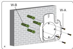
Place concrete anchors (W-B) in each hole. Tap each anchor flush with the wall using a hammer. Mount the wall mount and fasten screws (W-A) using a Phillips screwdriver.
