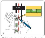
Using a level, mark the centerline of the stud.
