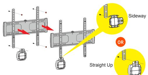
Choose the appropriate screws (M-A/ M-B/ M-C/ M-D/ M-E), washers (M-F/ M-G/ M-H), and spacers (M-I) if necessary, according to the type of your TV mount. Attach the Apple TV Wall Mount to the TV Wall Mount using a Phillips screwdriver.
