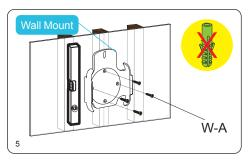
Using a Phillips screwdriver, mount the wall mount and fasten with the provided screws (W-A).
