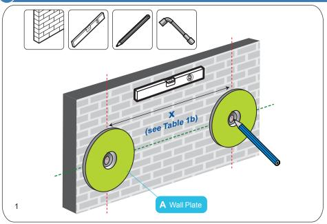
Hold the wall plate (A) as a template against the wall where you want to install your TV, mark two holes for drilling.
