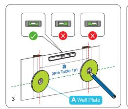
Using the wall plate (A) as a template, mark two holes for drilling on the centerline of the stud.
