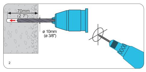
Using a power drill and a 3/8" masonry drill bit, drill mounting holes of 3/8" (10 mm) diameter and 2.7" (70 mm) depth at the marked locations in the previous step.
