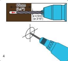
Using a power drill and 3/16" drill bit, drill pilot holes of 3/16" (4.5 mm) diameter and at least 2.5" (65 mm) depth.
