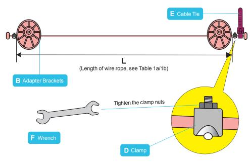
To adjust length of wire rope, loosen nuts of clamp (D), adjust wire rope length as necessary and re-tighten the clamp nuts using wrench (F).
