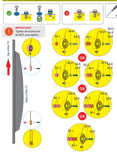
Choose the appropriate screws, washers, and spacers (if necessary) according to the type of your TV and tighten the adapter brackets (B) and the kickstands (C) to the back of the TV using a Philips screw driver.
