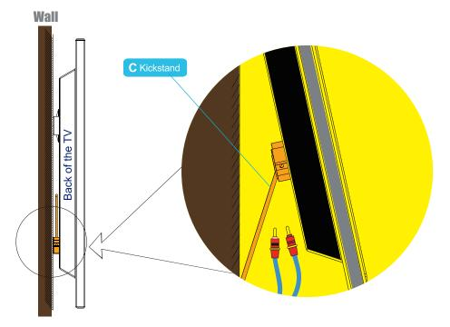
Fold out the kickstands to access the cables behind the TV. Once all cables are installed, unfold the kickstands.
