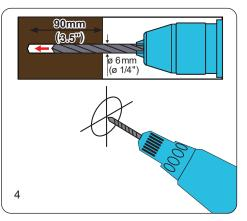
Using a power drill and 1/4" drill bit, drill pilot holes of 1/4" (6 mm) diameter and at least 3.5" (90 mm) depth.
