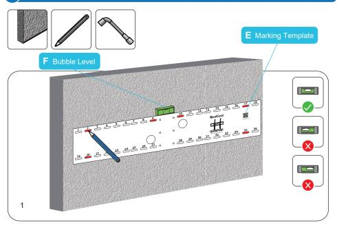
Hold the marking template (E) provided against the wall where you want to install your TV, mark six holes for drilling.
