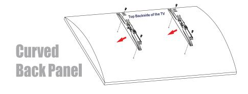
Choose the appropriate screws, washers, and spacers (if necessary) according to the type of your TV and attach adapter brackets (B and C) to the back of the TV using a Phillips screwdriver.
