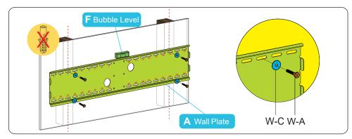
5 Mount the wall plate (A) and tighten it with the provided lag bolts (W-A) and D8 washers (W-C) using a socket wrench.
