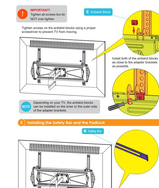
Insert the safety bar onto the rail (at the bottom of the wall plate) to secure.
