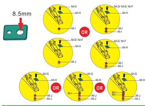
f 4 Hooking the TV onto the Wall Plate
