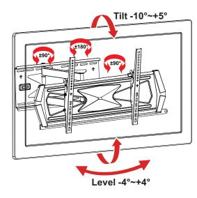
Adjust to the desired position by tilting  $-10^{\circ}$ +5°, swiveling  $-90^{\circ}$ +90°,  $-180^{\circ}$ ++180°,  $-90^{\circ}$ +90° at three pivot points and by leveling  $-4^{\circ}$ ++4°.
