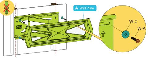
5 Mount the wall mount (A) and tighten it with the provided lag bolts (W-A) and D6 washers (W-C) using a socket wrench.
