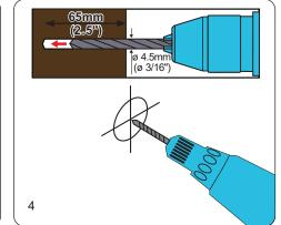
Using a power drill and 3/16" drill bit, drill pilot holes of 3/16" (4.5 mm) diameter and at least 2.5" (65 mm) depth.
