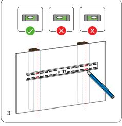
Using the marking template (C) provided, mark four holes for drilling on the centerline of the stud. Using a level, mark the centerline of the stud.
