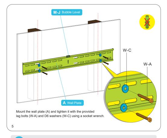
NOTE Do NOT use power drill and do NOT over tighten the lag bolts.
