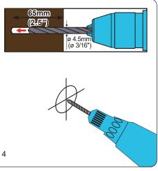
Using a power drill and 3/16" drill bit, drill pilot holes of 3/16" (4.5 mm) diameter and at least 2.5" (65 mm) depth.
