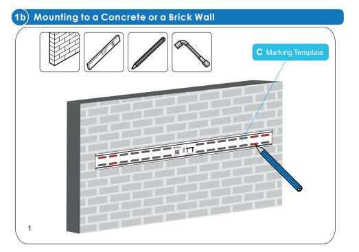
Hold the marking template (C) provided against the wall where you want to install your TV, mark six holes for drilling.
